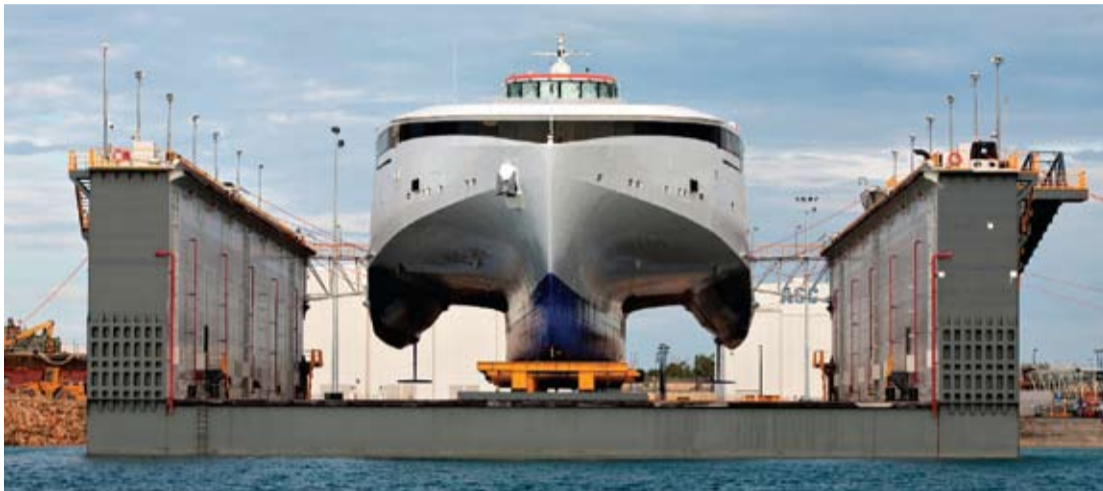
The AMC floating dock is the only dock in WA capable of docking the new Austal trimaran which has a width of 27m.
